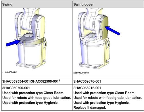
Details about the differences between swing 3HAC059554-001 and swing 3HAC082506-001, see Appearance description on page 890 and Spare part versions for the swing on IP40/IP67 robots on page 896.
