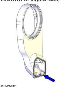
For robots with protection class IP67 For robots with protection type Foundry Radial sealing: 3HAC024865-001 **Plus**
