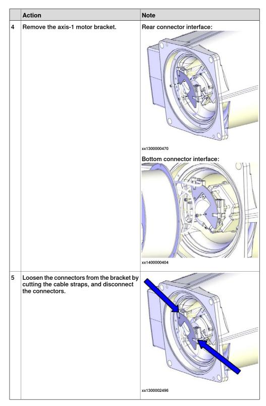
Removing the cable package from the base
